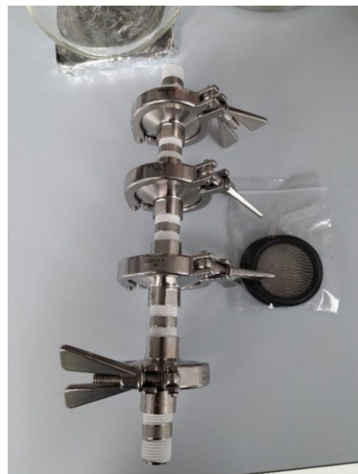
Sampling device compliant with the delegated act (EU 2020/2184) for the sampling of microplastics in drinking water. The left image shows the device connected to a faucet. The right figure displays the device along with the supporting meshes that hold the filters.
