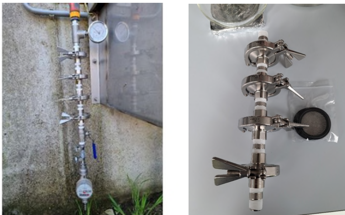
Figure 1: Cascade of four filters: two primary filters (a: 100\ \mu\text{m} , b: < 20\ \mu\text{m} ) for collecting suspended particles; two secondary filters (c: 100\ \mu\text{m} , d: < 20\ \mu\text{m} ) for procedure blanks. Materials used for this setup can be found in the supplementary information.
