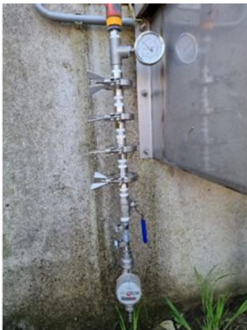
Sampling device compliant with the delegated act (EU 2020/2184) for the sampling of microplastics in drinking water. The left image shows the device connected to a faucet. The right figure displays the device along with the supporting meshes that hold the filters.
